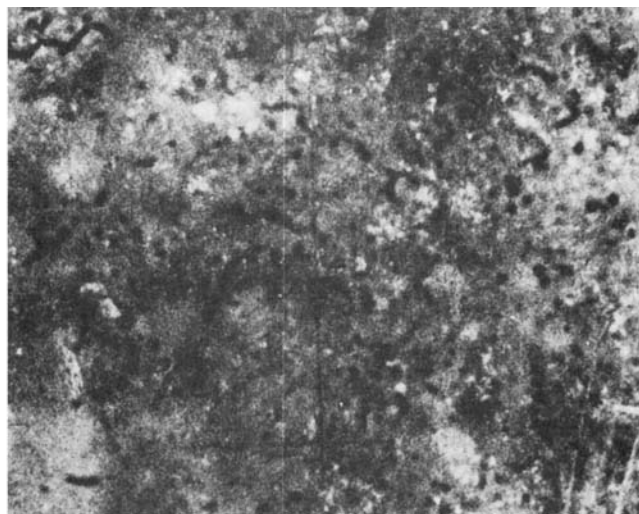
Figure 13 —Photomicrograph of cation-exchange resin compact after 4 hr of exposure to 100% relative humidity at 37°.
