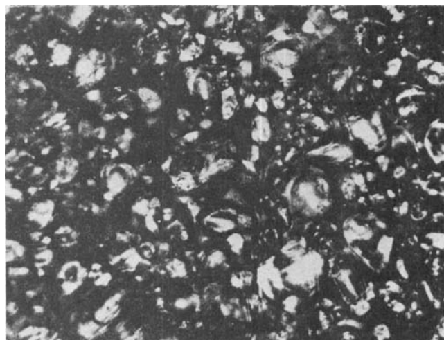
Figure 9 —Photomicrograph of sodium starch glycolate compact after 2 hr of exposure to 100% relative humidity at 37°.
